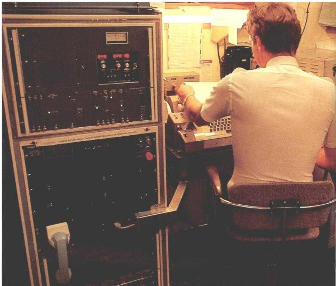
*High-speed data*—a new tariffed service was offered this year for ships with appropriately equipped terminals to transmit data at 56 kilobits-per-second in the ship-to-shore station. A voice-band data circuit is available for coordination with the ship during simplex 56 kbps transmissions, as required by the user.
